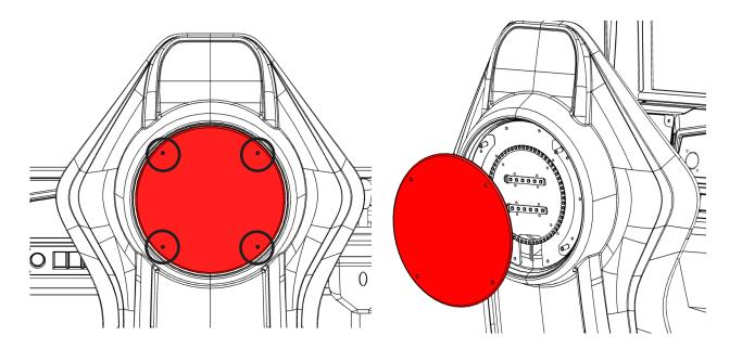
Remove and replace any faulty LED strips
