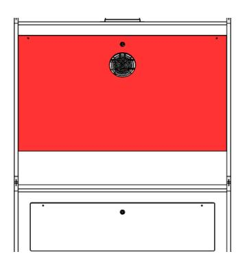
Remove the (3) M4 fixings highlighted
