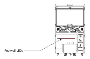
Remove the (2) M4x25 HEX KEY MSCR located at either end of the FOOTWELL LIGHTING COVER. Locate the LED strip and carefully peel away from the surface
