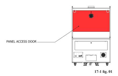
2 Unlock back panel by using key provided (keyhole labelled)
