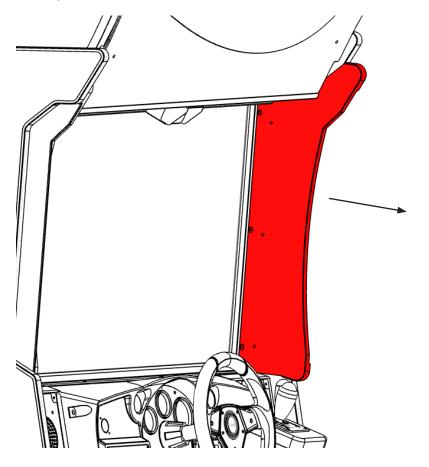
Replace the faulty LED strip on the inner side of INNER PANEL
