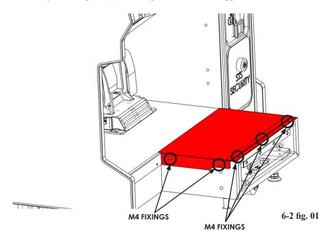
Align the Monitor Cab and Seat Cab. Connect the harnesses between the ASSY SEAT CAB and the ASSY MONITOR CAB
