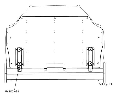
Secure the BILLBOARD BUMPER in place by inserting either the left or right side, then gently bending the bumper into position on the opposite side. Secure with (2) M4x50 fixings (1 on each side)
