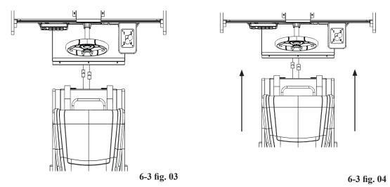
Once the SEAT CAB and MONITOR CAB are together, secure them using (4) M8 fixings in the positions illustrated below
