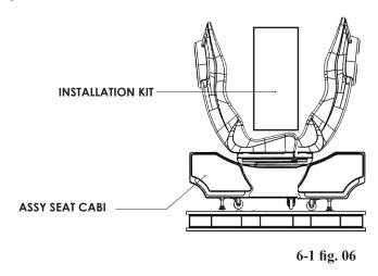
Remove the ASSY SEATS from the pallet using adequate lifting equipment. Failing to use such equipment may result in damage to components or personal injury.
