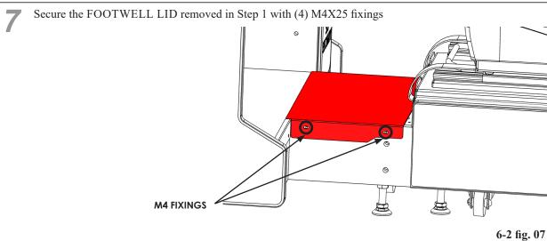
Secure the FOOTWELL LID SASH removed in Step 1 with (3) M4X25 fixings
