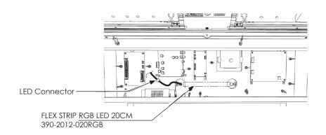
Carefully pull the LED STRIP through the access hole and discard. Fit a NEW LED STRIP by following these instructions in reverse order
