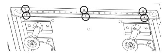
Remove and replace faulty LED strip
