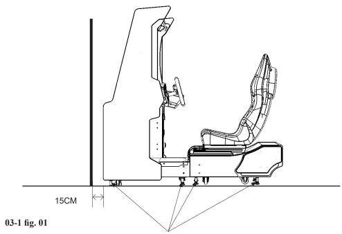
Ensure that all of the 8 adjusters are in contact with the floor. Provide a gap at the back of the cabinet ot no less than 15cm.
