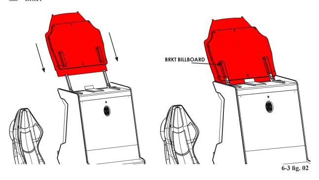
Secure the BILLBOARD in place using (2) M6X25 fixings on each bracket
